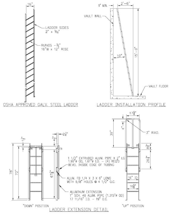
Figure 6—Ladder Fabrication and Orientation Details
