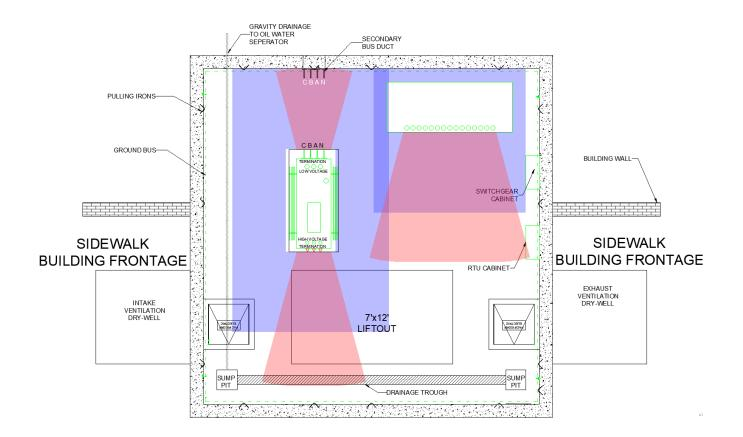
Figure 14—Below-Grade Vault, Top View
