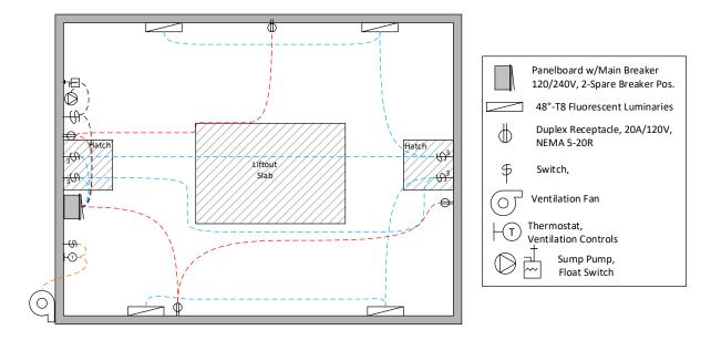
Figure 10—Example Station Service Electrical Plan Below-Grade Vault
