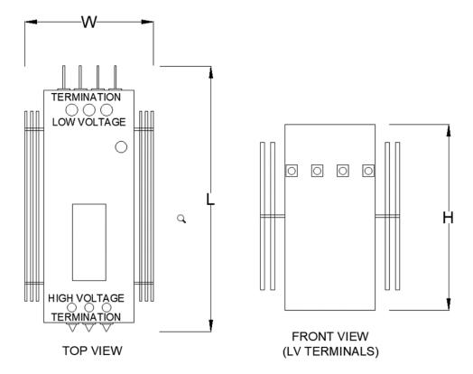
Figure 19—Three-Phase Submersible Transformers
