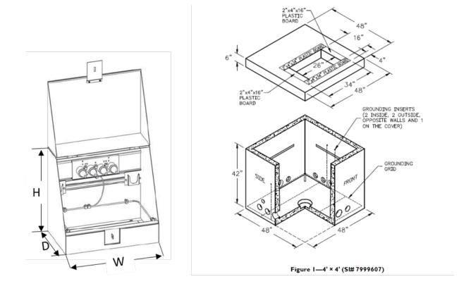
Figure 22—Single-Phase Sectionalizing Cabinet and Vault
