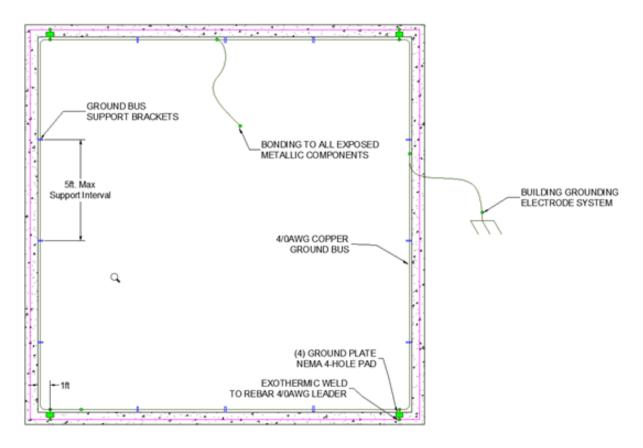
Figure 11—Example Vault Grounding and Bonding Diagram
