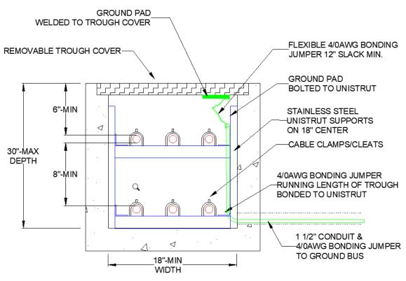
Figure 13—Example Primary Cable Trough Two Circuits
