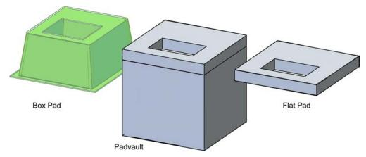
Figure I—Equipment Bases
