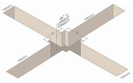
Figure 73—Excavation Dimensions – Secondary Box
