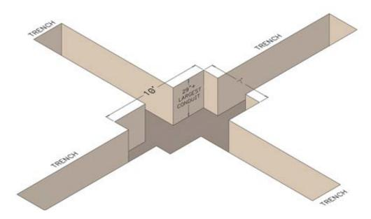
Figure 50—Excavation Dimensions - Three-Phase Sectionalizing Cabinet
