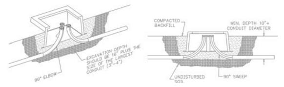
Figure 74—Top View/Side View - Secondary Box
