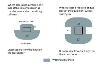
Figure 33—Working Clearances to Pad-Mounted Equipment
