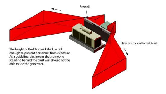
Figure 35—Typical Firewall
