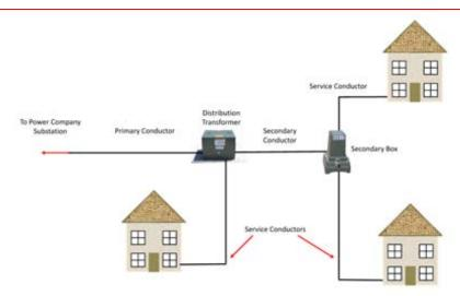
Figure 2—Primary, Secondary, and Service Conductor Schematic
