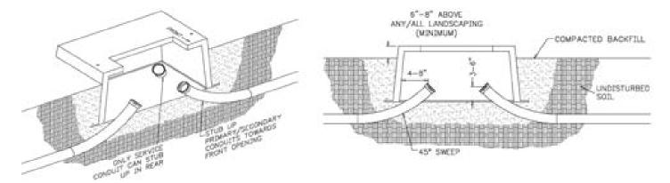
Figure 46—Top View/Side View - Single-Phase Sectionalizing Cabinet Box Pad
