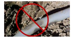
Figure 21—Field Altered Sweep - Damaged PVC
