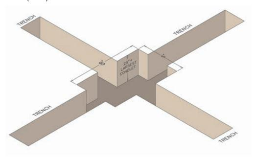
Figure 45—Excavation Dimensions - Single-Phase Sectionalizing Cabinet
