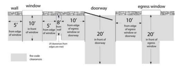
Figure 34—Clearances Between Equipment and Structures
