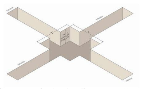
Figure 56—Excavation Dimensions - Single-Phase Transformer
