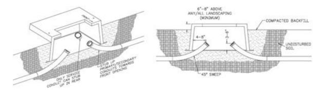
Figure 57—Top View/Side View-Single-Phase Transformer Box Pad
