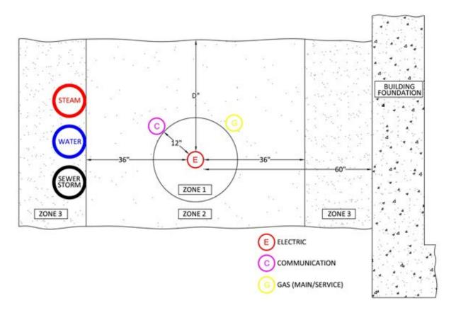
Figure 8—Separation of Paralleling Lines and Structures
