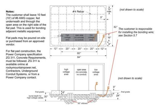
Figure 6 I — Dimensions and Installation of a Three-Phase Transformer Flat Pad Notes:
