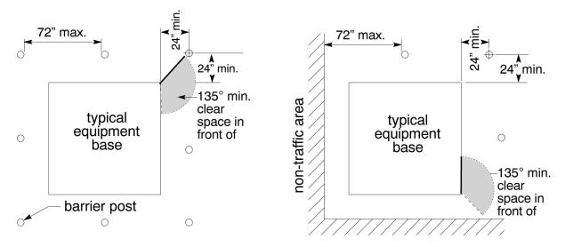
Figure 39-Barrier Post Layout and Clearances
