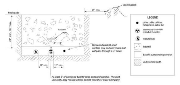
Figure I I—Joint Use Secondary Trench
